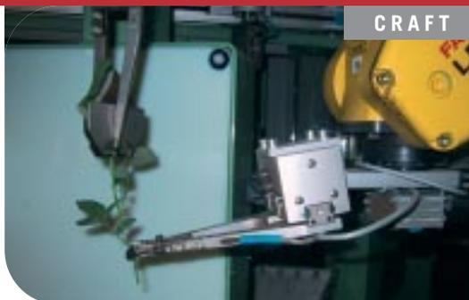
section of stem, and planting it in a pot – is all done manually. Mr Rombouts had the idea of using a robot to do this laborious and monotonous work.
